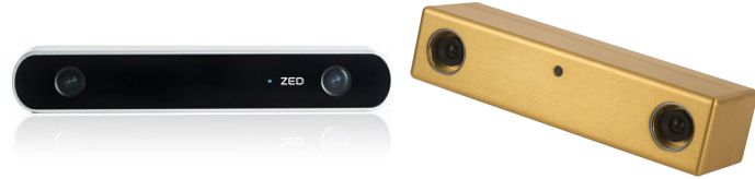
Stereo cameras (passive & fast but dependent on texture)
