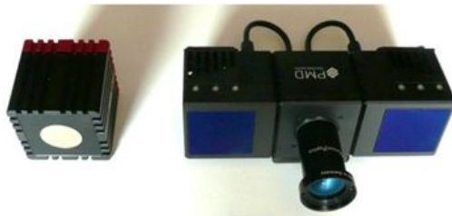
Time of flight cameras (fast but not as accurate/robust)
